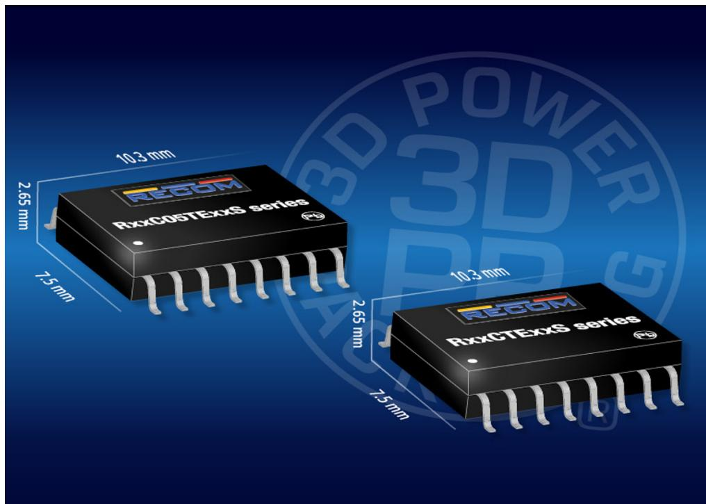
RECOM has extended its range of dc-dc converters housed in a low-profile SOIC-16 package.
